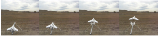
Figure 4. Plane-A-Pult Automatic Aircraft Launcher performing a fully autonomous launch.
