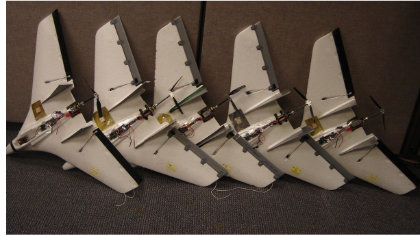
Figure 5. Our first flock of 5 MAVs. The design of each MAV is relatively simple, so scaling to produce larger flocks can be quickly achieved.
