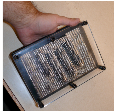
Figure 1. PinPoint toy with the impression of a human hand rendered via moving physical pixels, or “moxels”.
