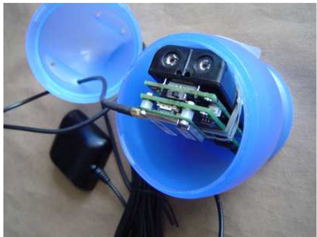
Fig. 2. MICAz node with the GPS board and batteries attached. The unit is protected with bubble wrap before closing the enclosure. The blue egg-like enclosure can be sealed to protect the unit, leaving just a small hole to get the GPS antenna connector inside the unit.
