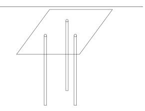
Figure 5. Plate articulation based on mounting a plate on three rods.
