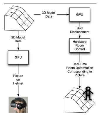
Figure 8. System Architecture
