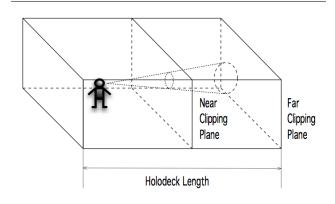
Figure 10. As the Holodeck PRE needs to render the complete physical area around the user, the adapted graphics program should not clip the immediate area around the user even if it is not visible to the user.
