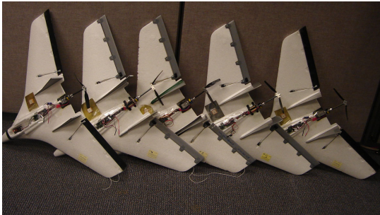
Figure 20: Our first SensorFlock of 5 MAVs. The design of each MAV is relatively simple, so scaling to produce larger flocks can be quickly achieved.
